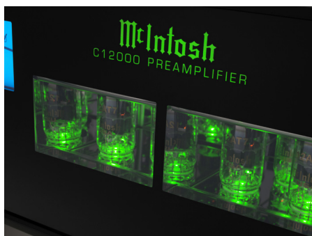
Top Left: C12000ST Preamplifier module. Top Right: C12000C Controller module. Bottom Left: The 12AX7A and 12AT7 vacuum tubes that power the high-level section are visible through the front of the C12000 Preamplifier module. Bottom Right: The four 12AX7A vacuum tubes that power the phono stage are visible from the top of the C12000 Preamplifier module.
