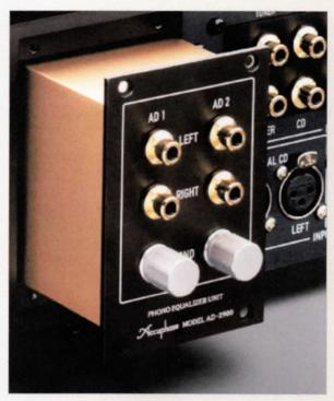
AD-2900 is the dedicated phono equalizer unit. Analog records can be reproduced with high quality by installing AD-2900 in a rear-panel slot. The AD-2900 features separate input circuitry for MC and MM cartridges to ensure optimum matching and realize outstanding S/N ratio. 2 sets of analog-player input jacks, the AD1 and AD2 are equipped, and their selections are switchable with the INPUT selector of pre-amplifiers.
